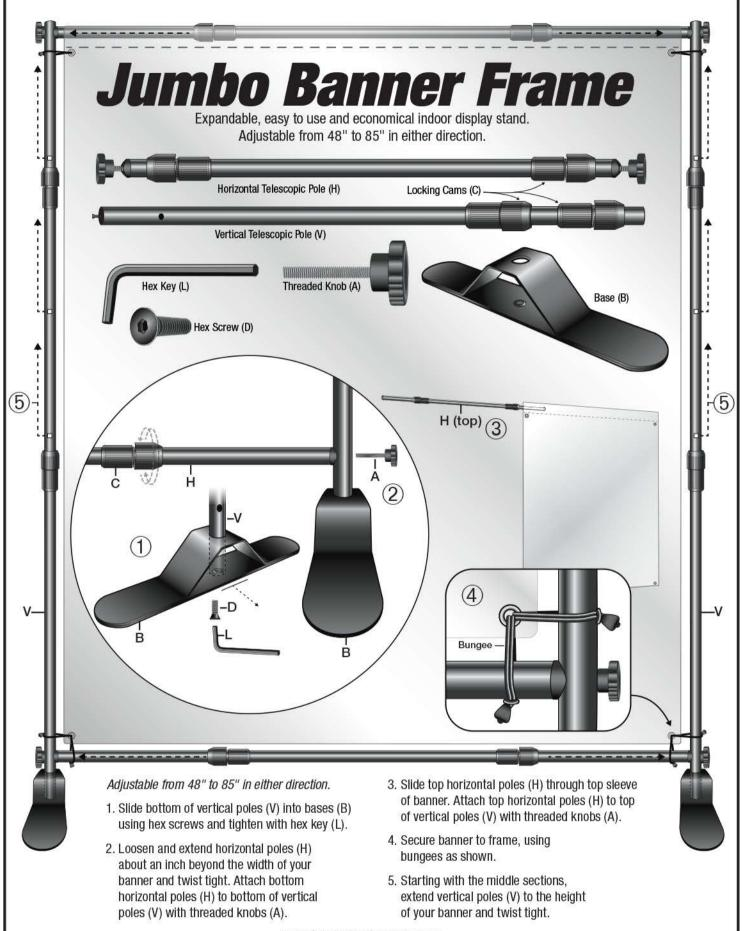
Do Not Over-Tighten Pole Cams.
